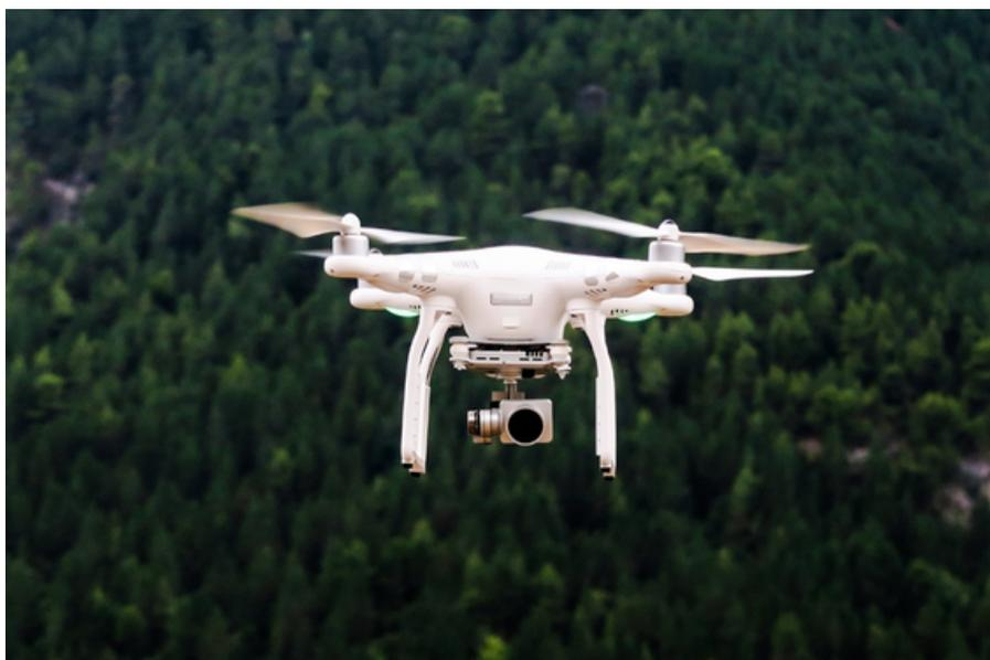
Fig.16 Exemple de drone VTOL (Vertical Take-Off and Landing)
